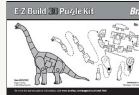
Exploded View shows how they are in relationship to each other using arrows to direct the sequence.
